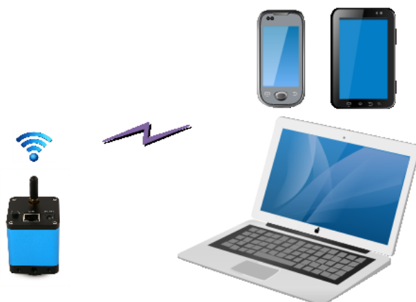
Figure 2 The PC or Mobile Device Connect to the Camera through WLAN AP Mode
