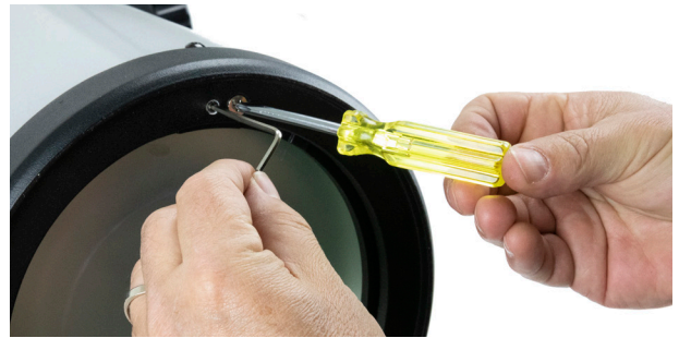
Figure 20: For the 8" Dob, there are three sets of push-pull screws in the mirror cell that adjust the tilt of the primary mirror. Loosen one screw in the pair and tighten the other to adjust the tilt.
