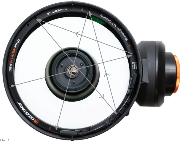
Fig 7 Alternately tighten the screws using a cross pattern as shown.
