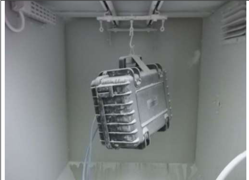
Photo 2: Set-up for the test to verify the protection degree IP 6X
