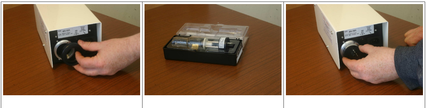
Fig: installing the Thorium-Argon lamp inside the calibration unit
