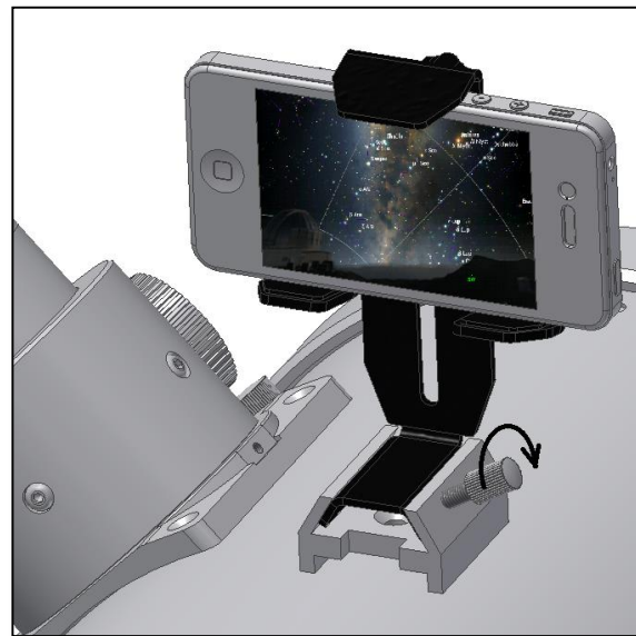
Figure 5. Slide the base into the Vixen-style finderscope base. Make sure to tighten the fixing thumbscrew.
